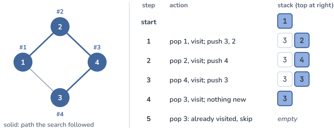
Figure 3.1.3 — Stack snapshots of iterative DFS from vertex 1 (only the component of 1 is shown). The search reaches 3 last, along 1 \rightarrow 2 \rightarrow 4 \rightarrow 3 , although 3 is a direct neighbour of 1.
